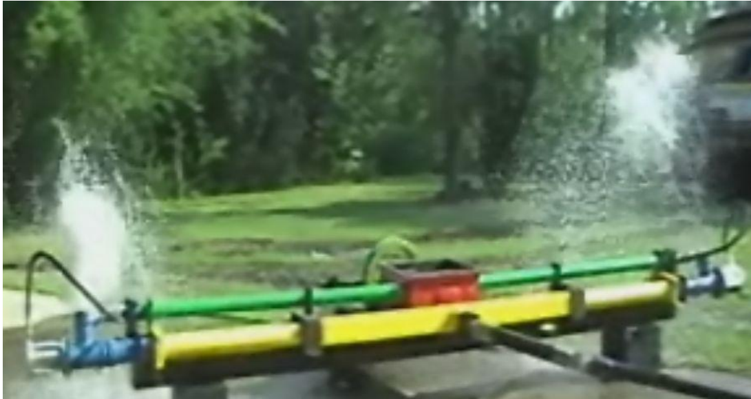
Figure 2. Linear Power, Ltd.'s Free-Piston Engine Being Driven by a Dual-Phase Mixture of Pressurized Gas and Water to Simulate the Effect of Gas-Lift Pumping of a Geothermal Well in order to Harness Its Kinetic Energy
